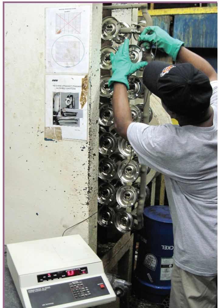
Eddy current instruments are rugged enough to use at the end of a plating line. Photo courtesy of Micro Metal Finishing.
