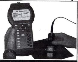
The Microderm<sup>CMS</sup> quickly measures lubricant coating weight on fe and non-fe substrates
